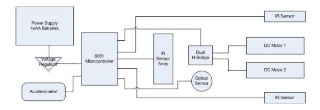
Figure 1: Component Diagram of Robotic Car Solution
