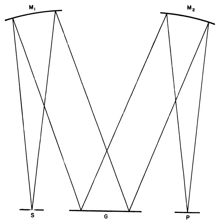
Fig. 7 The Lunar and Planetary Laboratory 10-foot Spectrograph (not to scale).
