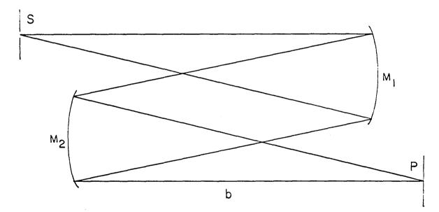
Fig. 6 The Czerny-Turner Design. The Angles Between the Mirrors and the Grating are Exaggerated.
