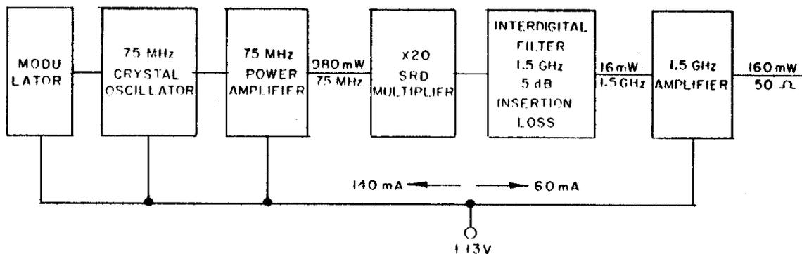
$$\eta = \frac{160 \text{ mW} \times 100}{13 \text{ V} \times 200 \text{ mA}} = 6.1 \text{ percent}$$
