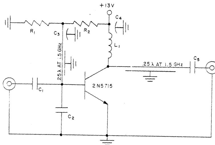
$C_3 = C_4 = 25$  pf EYELET FEED THRU CAPACITOR
