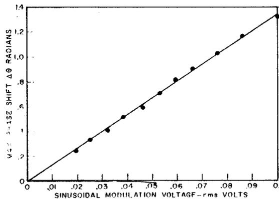
**Fig. 4 - Modulation Sensitivity**
