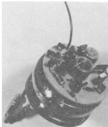
**Fig. 10 - L-Band Transmitter**
