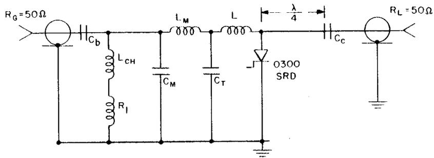
$C_b = 62 \text{ pf}$      $R_1 = 18 \text{ ohms}$      $L_{CH} = 1.5 \mu\text{h}$  MOLDED CHOKE
