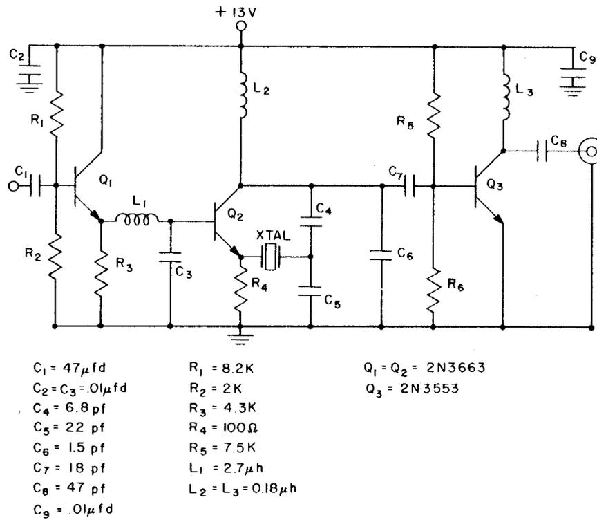
**Fig. 2 - Modulator, 75-MHz Crystal Oscillator, and Power Amplifier**
