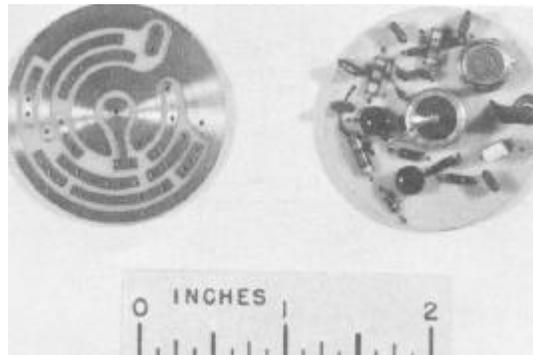
**Fig. 3 - Modulator, 75-MHz Crystal oscillator, and Power Amplifier**
