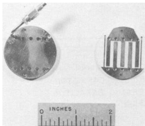
**Fig. 7 - 1.5 GHz Interdigital Filter**
